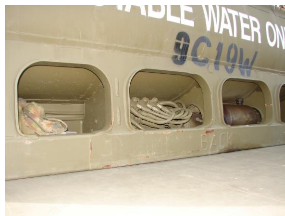
Figure 36-6: Water Tank Self Deployable 3000 L Stowage and Fuel Areas
