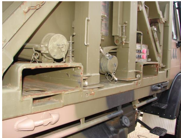
Figure 36-5: Water Tank Self Deployable 3000 L Forklift Tynes Slots
