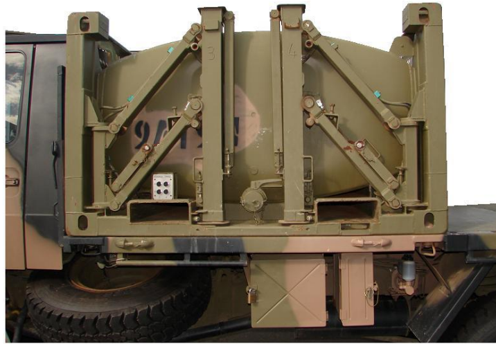
Figure 36–2: Water Tank Self Deployable 3000 L Packed For Transport
