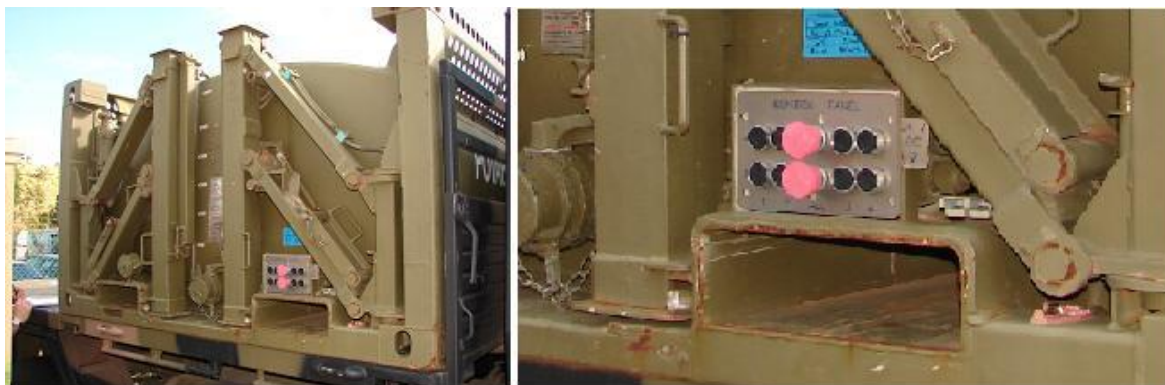
Figure 36–4: Water Tank Self Deployable 3000 L Control Panel
