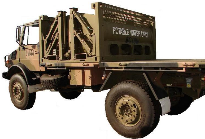
Figure 36–3: Water Tank Self Deployable 3000 L Truck Mounted
