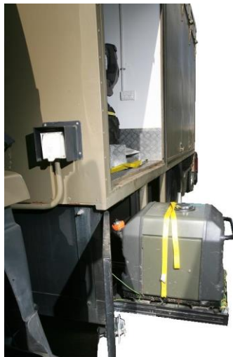
Figure 45-3: DMV's Portable Generator Compartment
