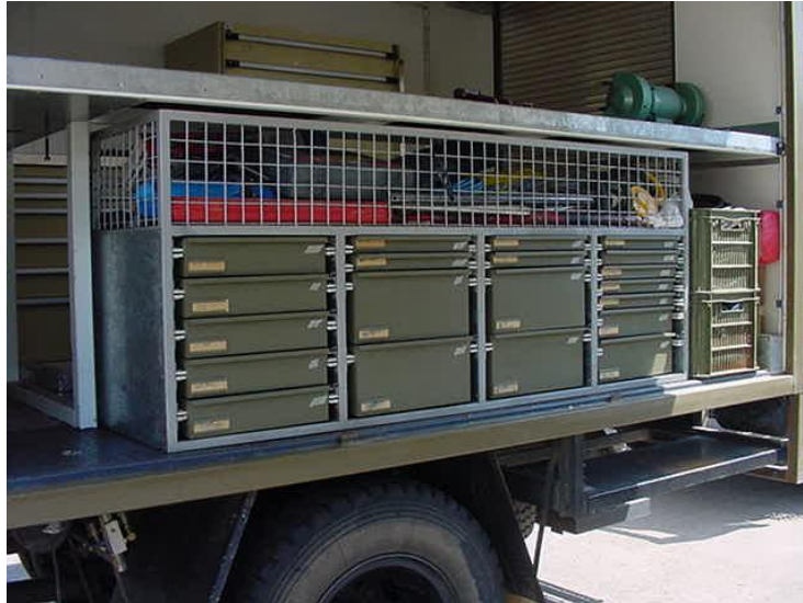
Figure 45-12: DMV's Rear Exterior Metal Drawer Storage
