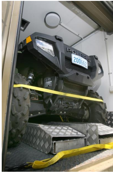
Figure 45-5: DMV's 4X4 All Terrain Vehicle Stowage Compartment
