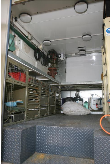
Figure 45-10: DMV's Rear Interior Metal Shelving Storage
