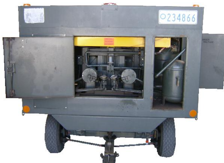
Figure 50A-4: TEC 300 AC Aircraft Air-conditioning Unit Condensers
