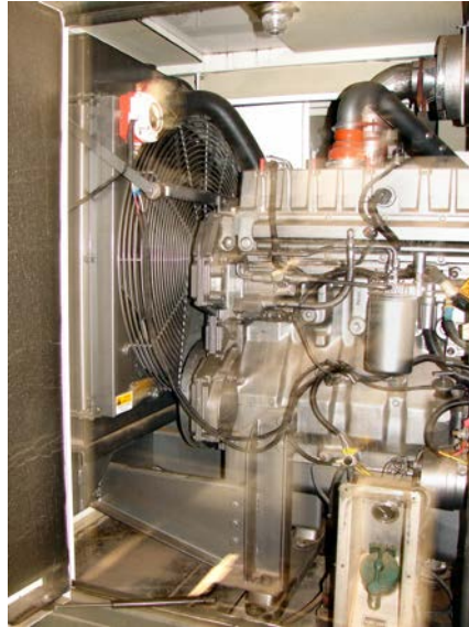
Figure 50B-5: 5080DE Aircraft Air-conditioning Unit's Radiator and Fan
