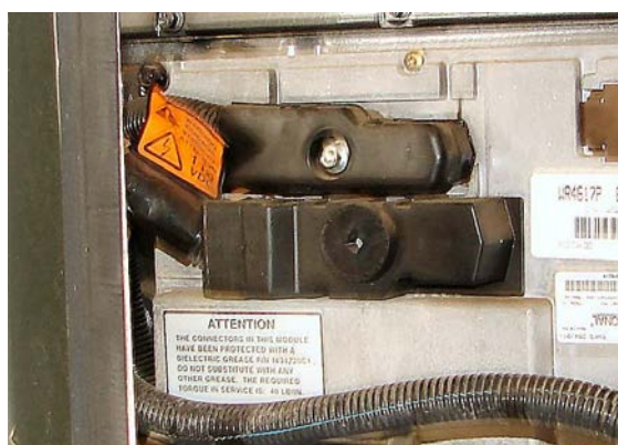
Figure 50B-3: 5080DE Aircraft Air-conditioning Unit's Engine Bay Computer
