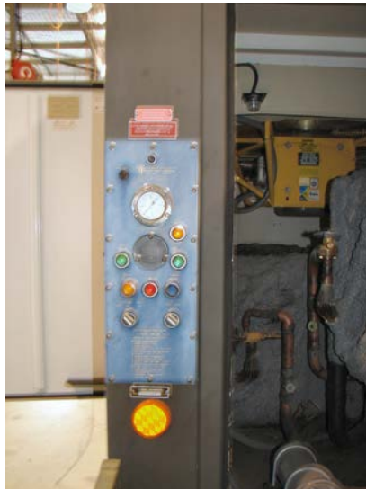
Figure 50B-12: 5080DE Aircraft Air-conditioning Unit's Operator Control Panel
