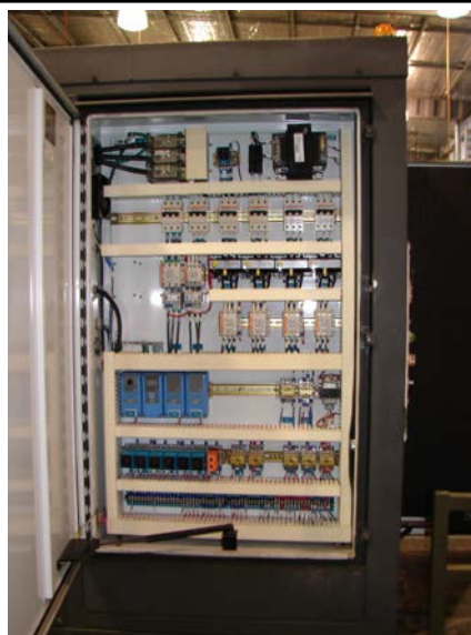
Figure 50B-10: 5080DE Aircraft Air-conditioning Unit's Electrical Circuit Box
