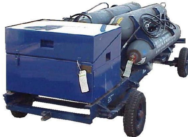
Figure 54–4: The Nitrogen Booster and Regulator Cabinet (NBRC)
