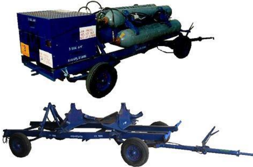
Figure 54–3: 4 Bottle Nitrogen Trailer Pre and Post De-rigging for Cleaning
